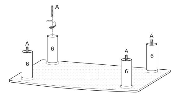
Screw long rods (A) into cylinders (6).
